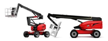
Our articulated (internal combustion engine and electric) and telescopic (internal combustion engine) models allow working heights from 12 to 28 m.
