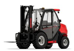
MC-X models. Working heights from 3.3 m to 5.5 m and lifting capacities from 1.8 t to 3 t.
